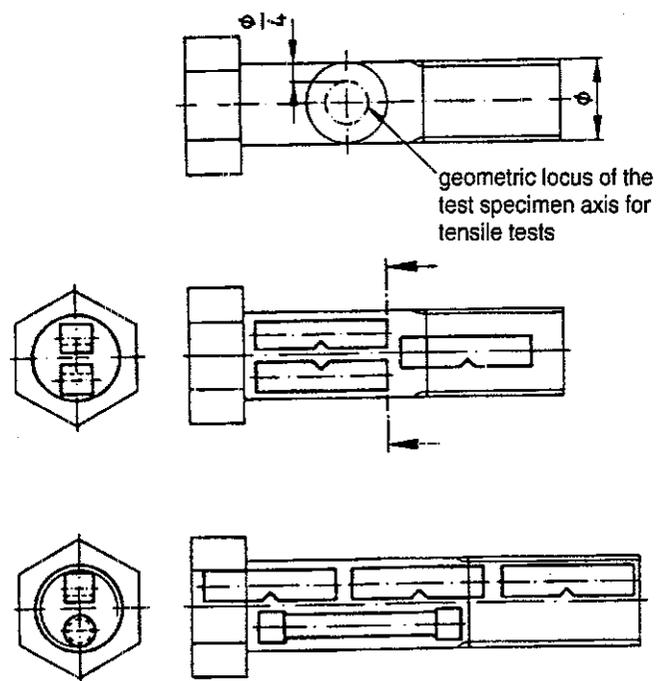
**Figure 9-1:** Specimen removal from bolt blanks with hot formed bolt head and subjected to subsequent quenching and tempering
