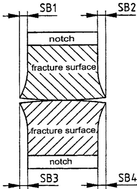
Figure D-1: Determination of the lateral expansion (SB) of broken notch bend test specimens
