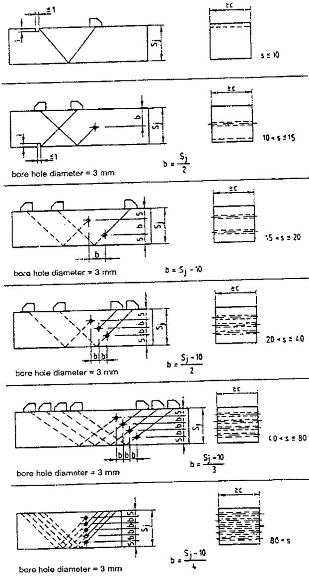
Figure B-1: Reference bodies for the sensitivity adjustments of the angle beam examination
