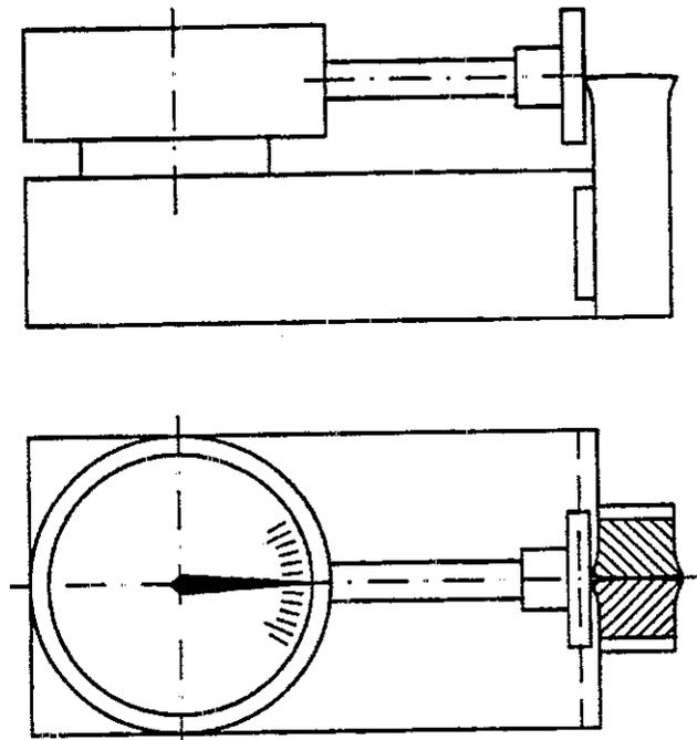
Figure D-2: Measurement principle for a simplified procedure for the determination of the lateral expansion (SB)
