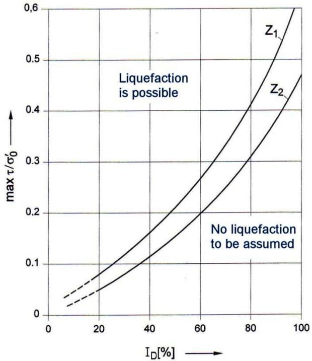
**Figure A-5:** Diagram for estimating the possibility of soil liquefaction
