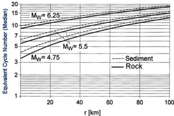
**Figure A-2:** Equivalent cycle number,  $N$ , as a function of the moment magnitude,  $M_W$ , and the shortest distance,  $r$  (km), from the epicenter
