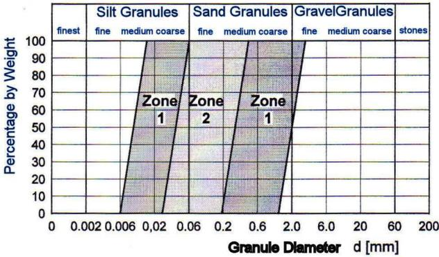
**Figure A-4:** Grain size distribution zones susceptible to liquefaction
