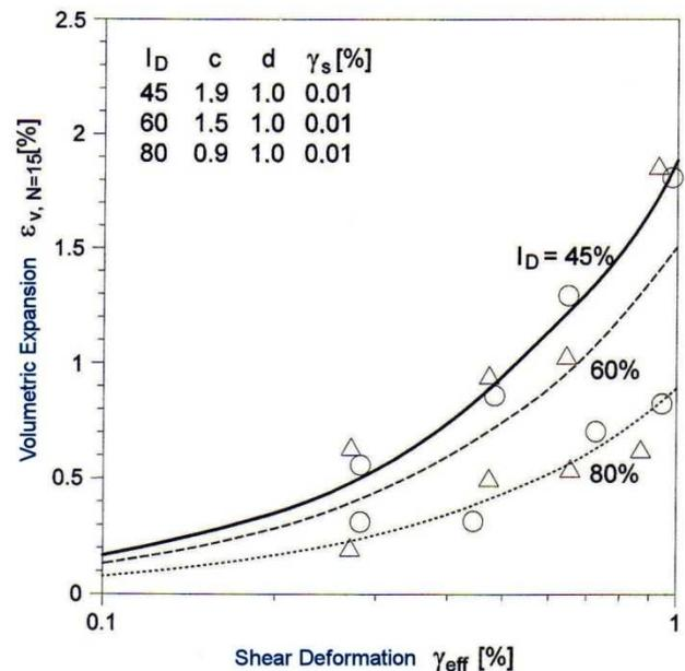
**Figure A-3:** Material model sand without fine grains –  $I_D = 45\%$ ,  $60\%$  and  $80\%$  (cf. [2])
