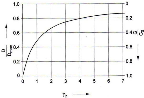
**Figure A-1:** Relationship between dynamic shear modulus, material damping and hyperbolic shear deformation
