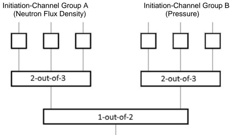
**Figure 4-2:** A possible schematic for the actuation of the reactor scram; it is caused by reactivity disturbances where two actuation criteria derived from different process variables (e.g., neutron flux density and pressure) are available and any secondary failures in data acquisition can be precluded.
