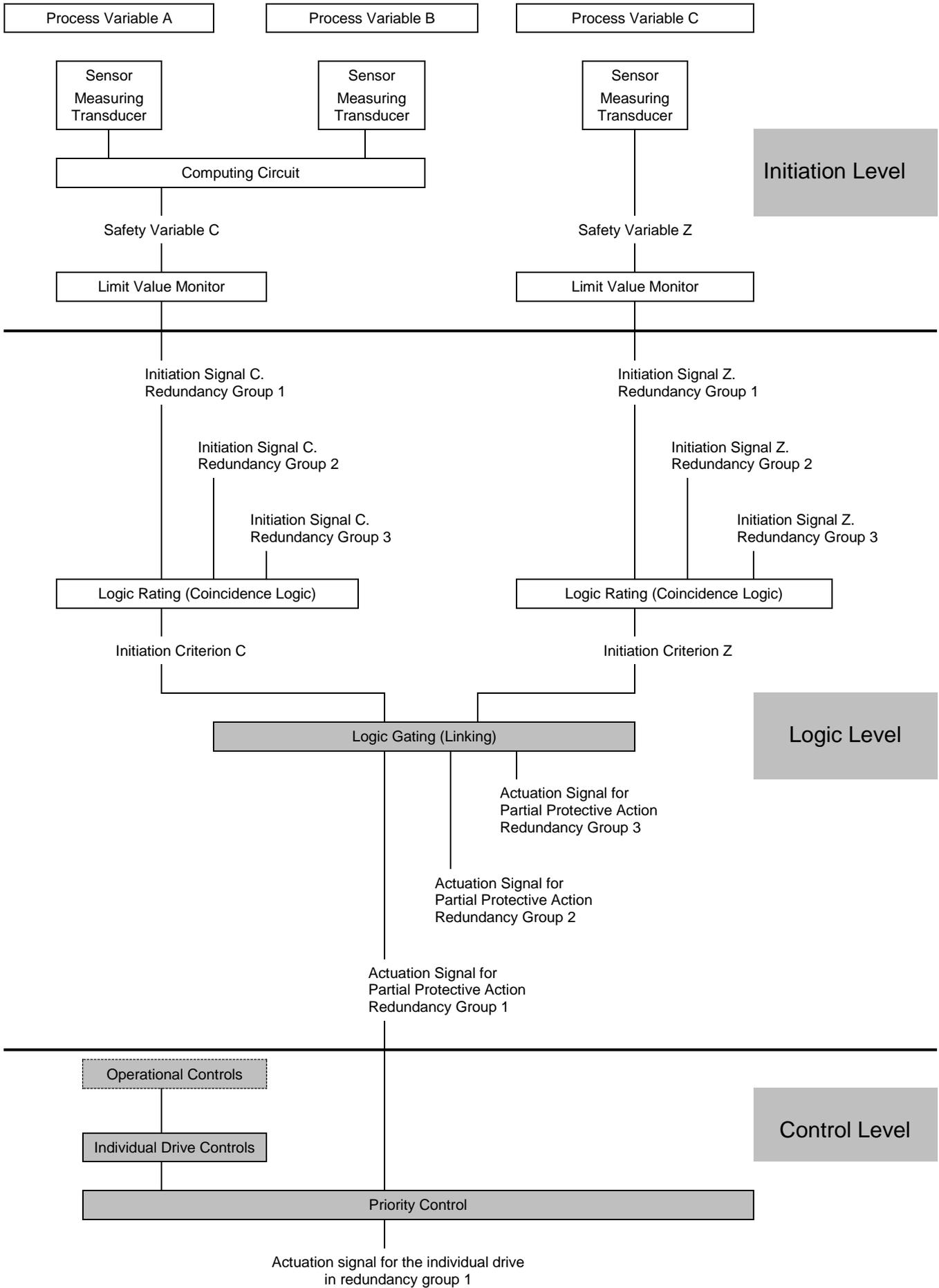
**Figure 2-1:** Exemplary correlation of the defined terms to the functional design of Cat A equipment
