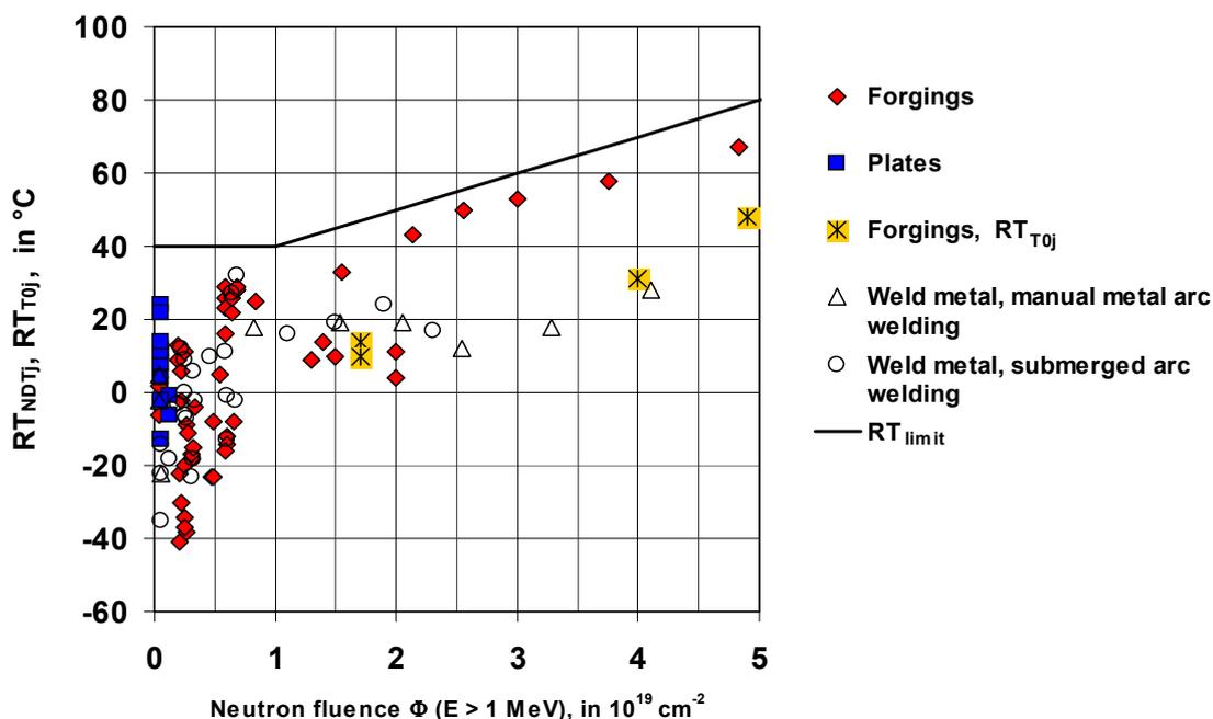
**Figure B-1:**  $RT_{NDTj}$ ,  $RT_{T0j}$  as a function of neutron fluence, results obtained on base materials and weld metals from irradiation surveillance programs in German reactor RPV (BWR and PWR); only weld metals with percent by mass of  $\text{Cu} \leq 0.15 \%$  and  $0.05 \% < \text{Ni} \leq 1.7 \%$ .
