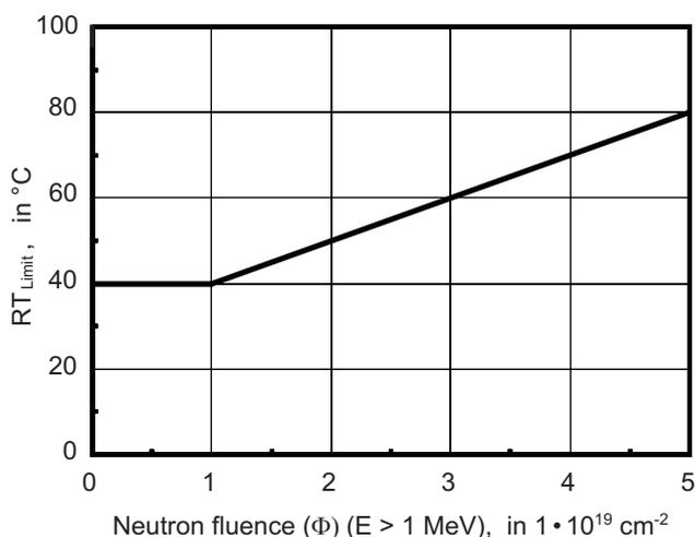
This limit value applies to neutron fluences (at neutron energies  $E > 1 \text{ MeV}$ ) equal to or greater than  $1 \cdot 10^{17} \text{ cm}^{-2}$  and for materials meeting the requirements of section B 5.1. At present, results are available for boiling water reactors amounting to neutron fluences (at neutron energies  $E > 1 \text{ MeV}$ ) of up to  $1 \cdot 10^{18} \text{ cm}^{-2}$ .
