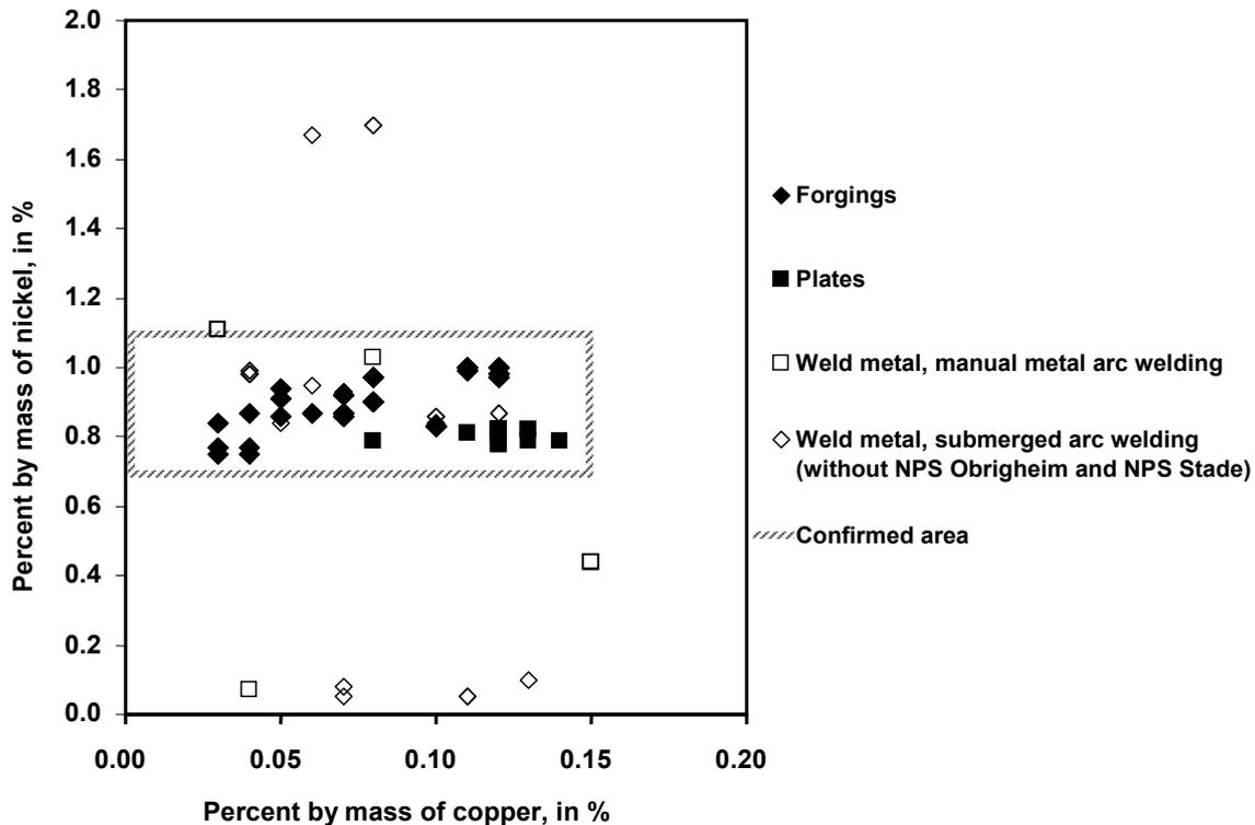
**Figure B-2:** Area of copper and nickel percentage by mass covered by results obtained from RPV irradiation surveillance programs
