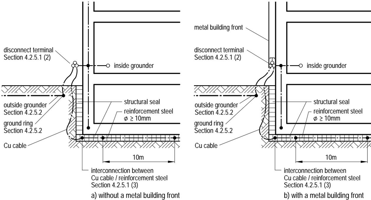
**Figure 4-2:** Interconnection of the foundation earth electrode in the case of buildings with an external structural seal
