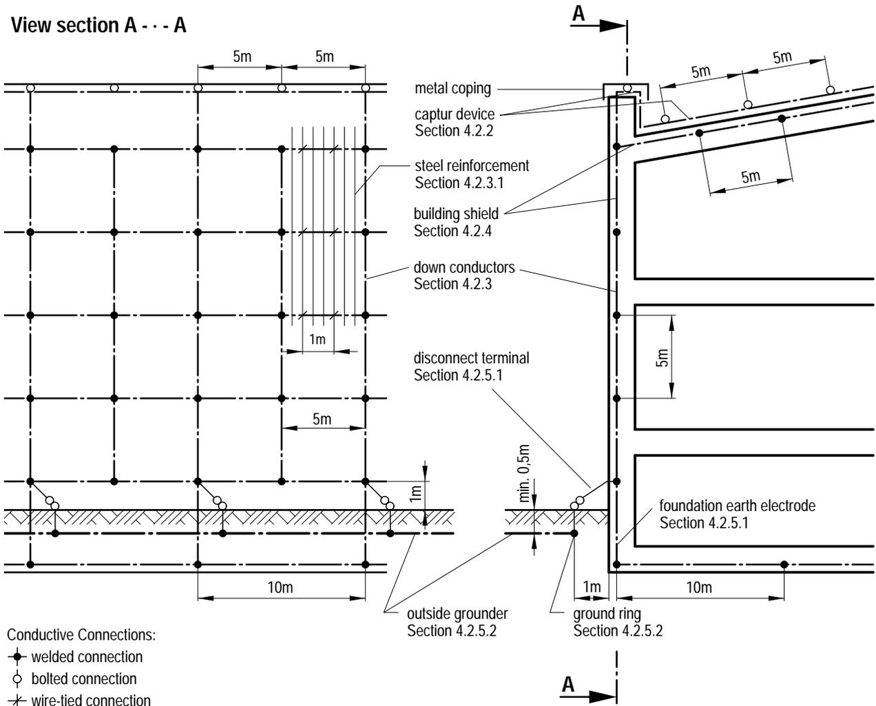
**Figure 4-1:** Reinforcement steel rods for the building shield in the case of buildings without a metal building front, and interconnection of the foundation earth electrode in the case of buildings without an external structural seal
