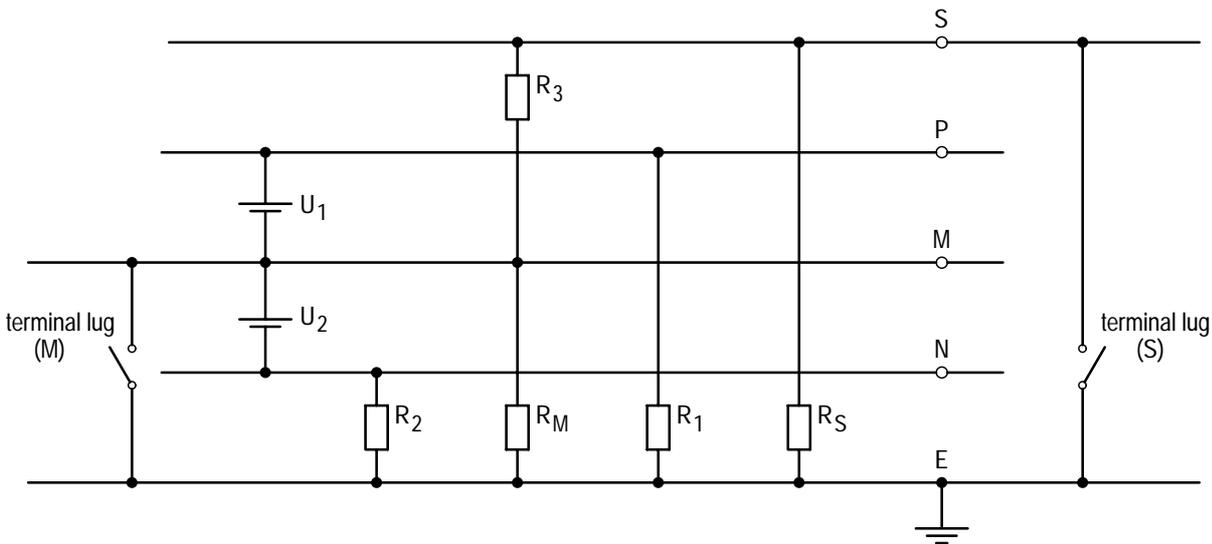
**Figure B-1:** Simplified circuitry of a 24-volt facility with a central grounding point
