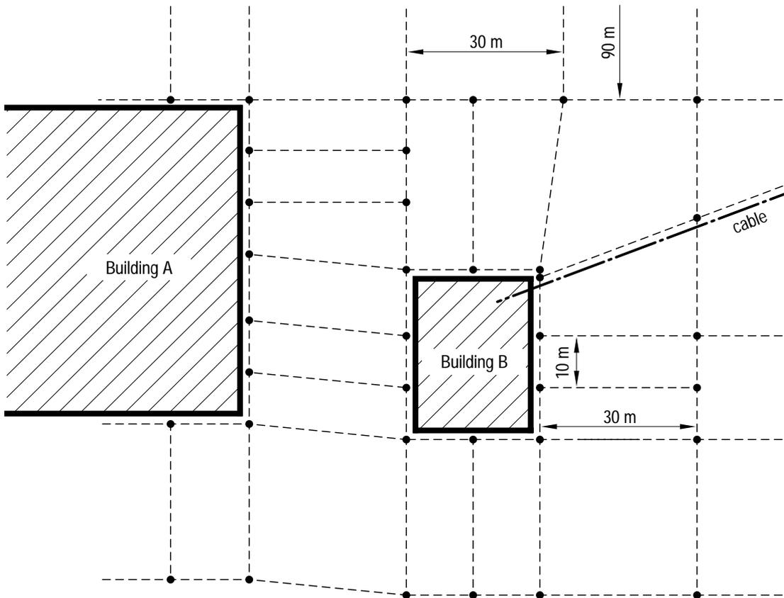
Figure 4-4: External grounding between buildings
