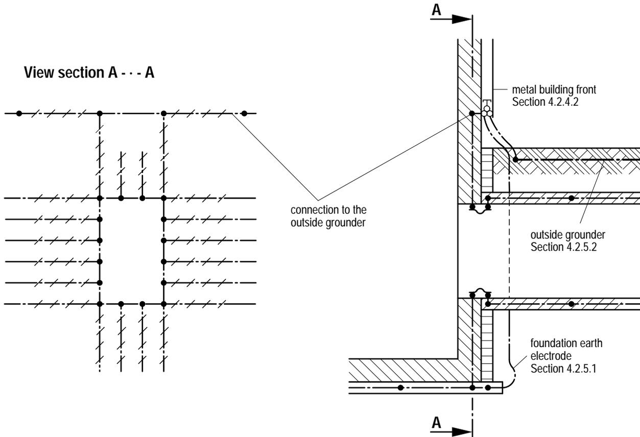
**Figure 4-6:** Cable duct, interconnection of the cable duct shield to the metal building fronts and to the foundation earth electrode in the case of an insulated foundation
