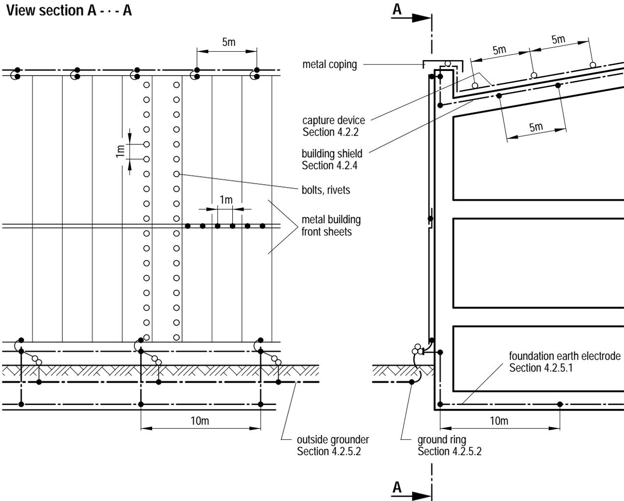
**Figure 4-3:** External lightning protection in the case of buildings with metal building fronts (height of lower lip less than 1 meter above ground) and without an external structural seal
