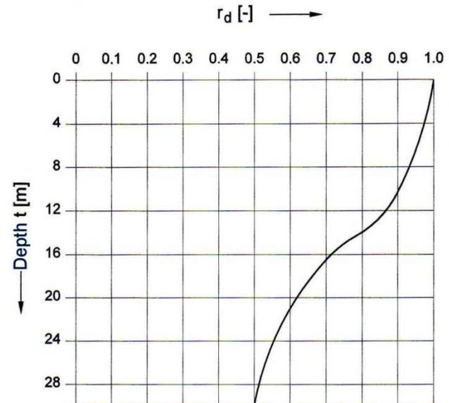
**Figure A-6:** Reduction factor,  $r_d$ , as a function of depth,  $t$
