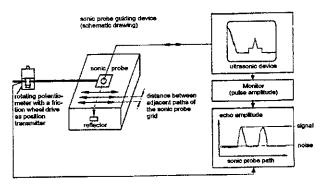
Figure B-11: Measurement device for employing focussing sonic probes for the determining the reflector size
