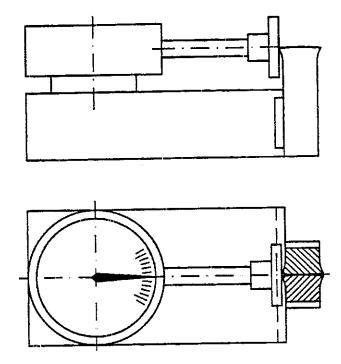
gure D-2: Measurement principle for a simplified procedure for the determination of the lateral expansion (SB)
