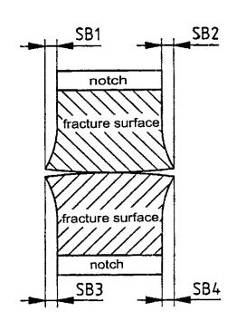
Figure D-1: Determination of the lateral expansion (SB) of brock- Figure D-2: en notch bend test specimens
